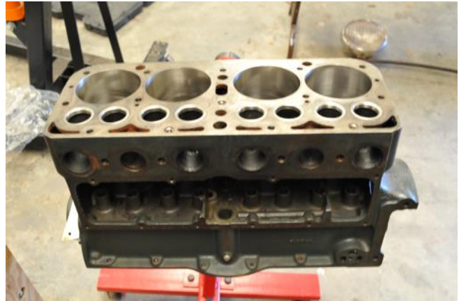
The engine block out of my 1930 Cabriolet, required crack repair, sleeved cylinder, new babbitt, and new valve seats.. Should run like a champion!
