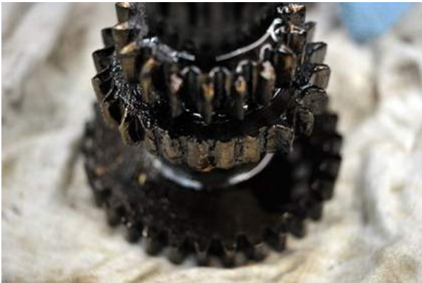
Figure 3: Notice the flattened or missing second gear up from the bottom. This is officially "junk".
