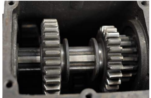
Figure 2: These original gears look pretty good and fit tight on the shaft "within tolerance".
