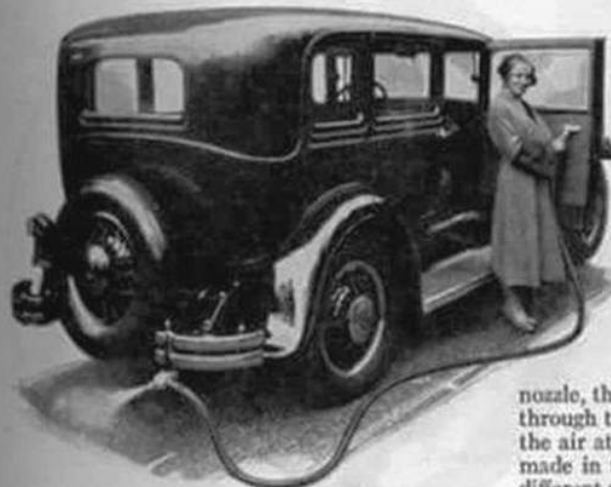
With the car's engine idling, gas from the exhaust creates a vacuum that cleans the cushions.
