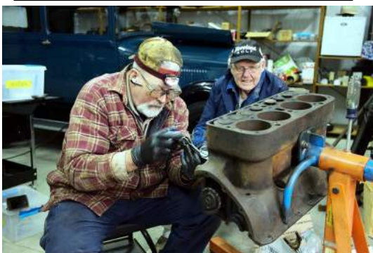
Eric and Noel hard at work in Guben's Garage. Eric tells us 'the block is a test block for when I first pour babbit bearings.' (photo by Greg Jones)
